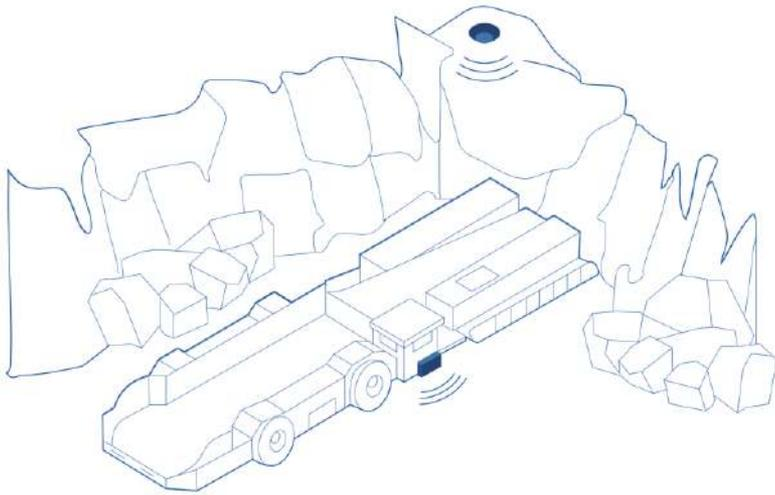
Similarly to the previous scenario, the BLE antennas are installed in industrial vehicles (dumpers, excavators, various loaders, bulldozers, etc.) and the Beacon in the various work areas. When the machines enter the area, the position of the vehicle is detected.
